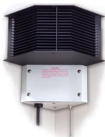
**CM15** is designed to mount in room corners with two keyhole slots at 7 ft. This fixture incorporates a GML500 lamp and covers 75 - 100 square feet. The CM15 fixture comes complete with an eight-foot power cord and an on/off switch. The louver restricts and concentrates the ultraviolet rays above eye level so **personnel can occupy the room** while the fixture is on.
