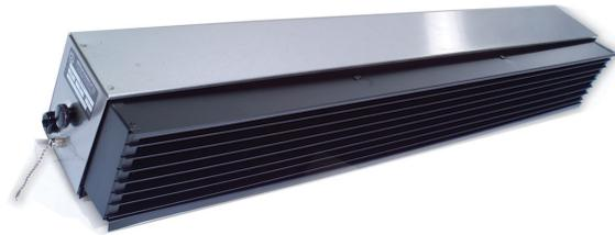
Models **TB-W** are designed to be wall-mounted to reduce upper air contamination. TB-W fixtures feature adjustable louvers to allow unlimited direction of the ultraviolet rays while protecting personnel and providing maximum germicidal irradiation. The units are constructed of high grade stainless steel with an alzak aluminum reflector.
